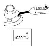
4. While holding the unit, press and release the ON-OFF Button. The radiometer will then provide a reading of the light intensity on the cradle display.
